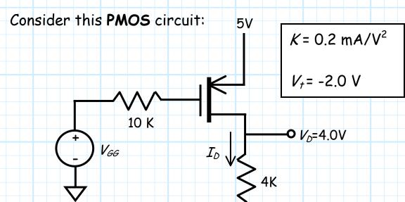
For this problem, we know that the **drain voltage**  $V_D$  = 4.0 V (with respect to ground), but we do **not** know the value of the voltage source  $V_{GG}$ .
